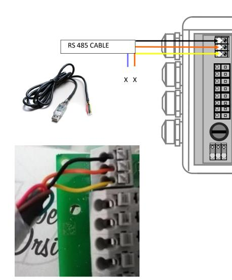
Connect the cable wires into the controller;
