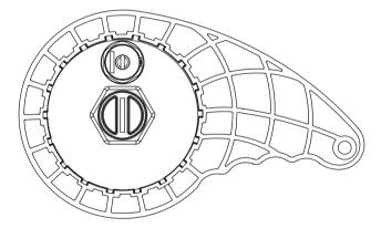
Before removing the filter screw cap drain the filter or open the air vent to relieve internal pressure in the filter pot.
