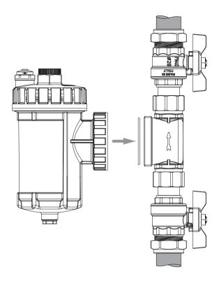
Present the filter to the connector block ensuring the air bleed is at the top and the drain plug is at the bottom.
