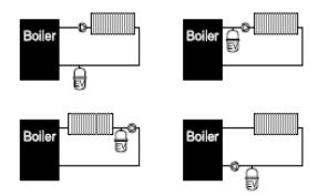
Check the pressure gauge when the system is cold to identify any pressure loss below the set point. A loss of pressure indicates either air venting or a system leak. Re-pressurise as required and continue to observe.
